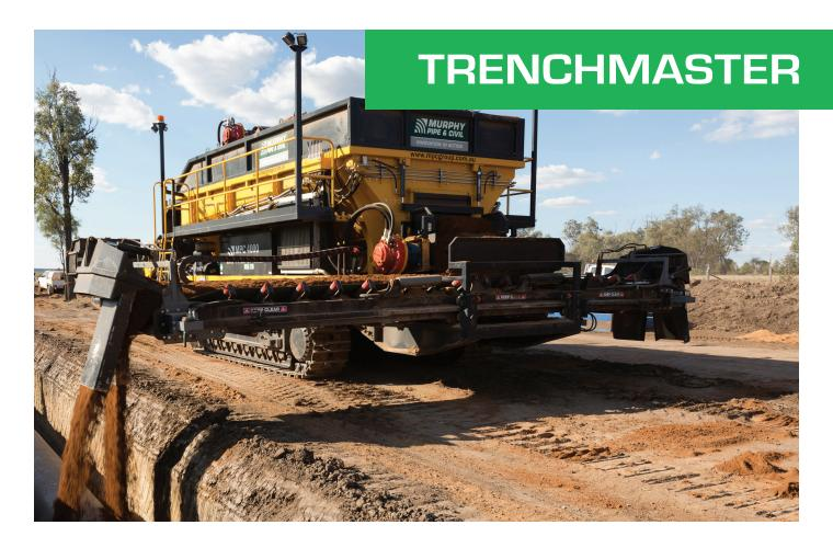
MPC Kinetic's constant pursuit for efficiency was a driver behind the company's in-house R&D team's concept, design and development of the Trenchmaster EF450 sand bedding machine. Apart from efficiency gains in bedding sand placement, the Trenchmaster EF450 also delivers increased safety benefits by eliminating the number of ground crew and machinery needed for this part of the pipeline construction process.
