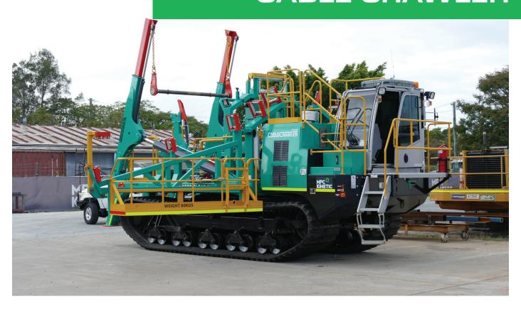
MPC Kinetic's innovative cable crawler is the fastest and safest method for installing High Voltage and Fibre Optic cable within the industry. The purpose-built machine provides clients with a cost-effective and safer solution for installing cables up to 110mm in diameter.
